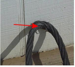
Damaged wire rope sling in shipping area
