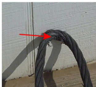
Damaged wire rope sling in shipping area
