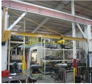
Jib crane load limits are not legible from ground
