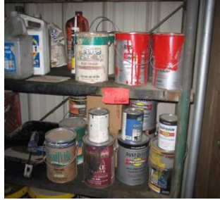
Paint shop could use two more flammable storage cabinets
