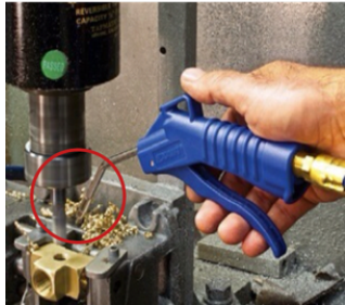
Non-compliant air nozzle
