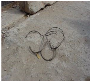
Defective wire rope sling in Yard
