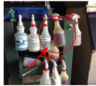
Secondary containers not properly labeled
