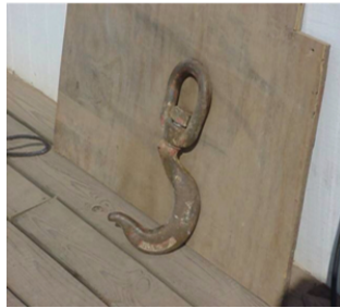
Defective lifting hook
