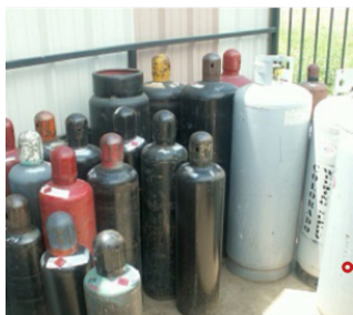
Example of cylinders NOT stored properly
