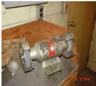
Grinder should be mounted to work bench and guards installed
