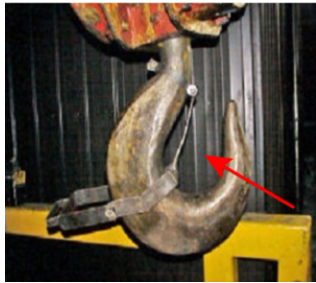
Safety latch is broken - East bay
