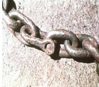
Defective chain sling in shop
