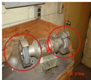
Guards not adjusted properly
