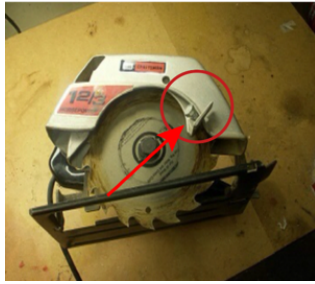
Bolt is being able send to bypass guard
