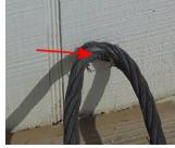
Defective wire rope sling in Yard Damaged wire rope sling in
