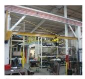
Jib crane load limits are not legible from ground
