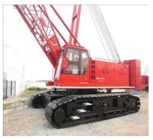
Radius guard is missing on this crane
