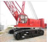
Radius guard is missing on this crane
