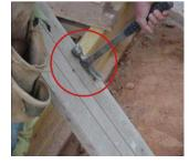
Nails were removed or bent down on several boards of scrap lumber
